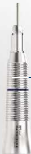
LB02 195 Straight Handpiece 1:1, blue External water via clip-on hose Max. 20.000 rpm For HP burs (Ø 2.35 mm) and disposable prophylaxis heads Intramatic® connection
