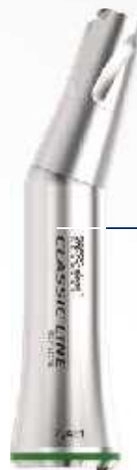
LC74L / LC74 395 / 345 Contra Angle Body with / without light 7,4:1, green With internal water Max. 5.406 rpm For MK-dent and KaVo® heads
